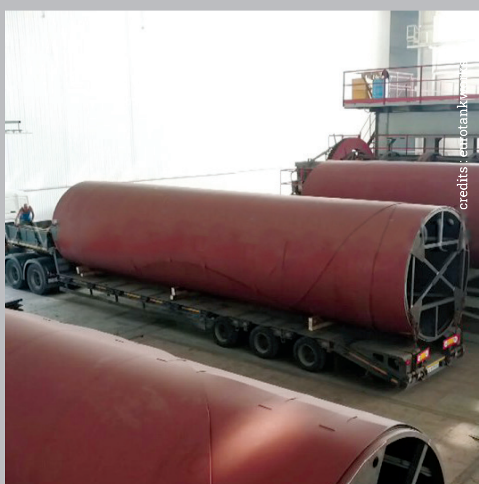
coiled tank sheets ready for transportation
