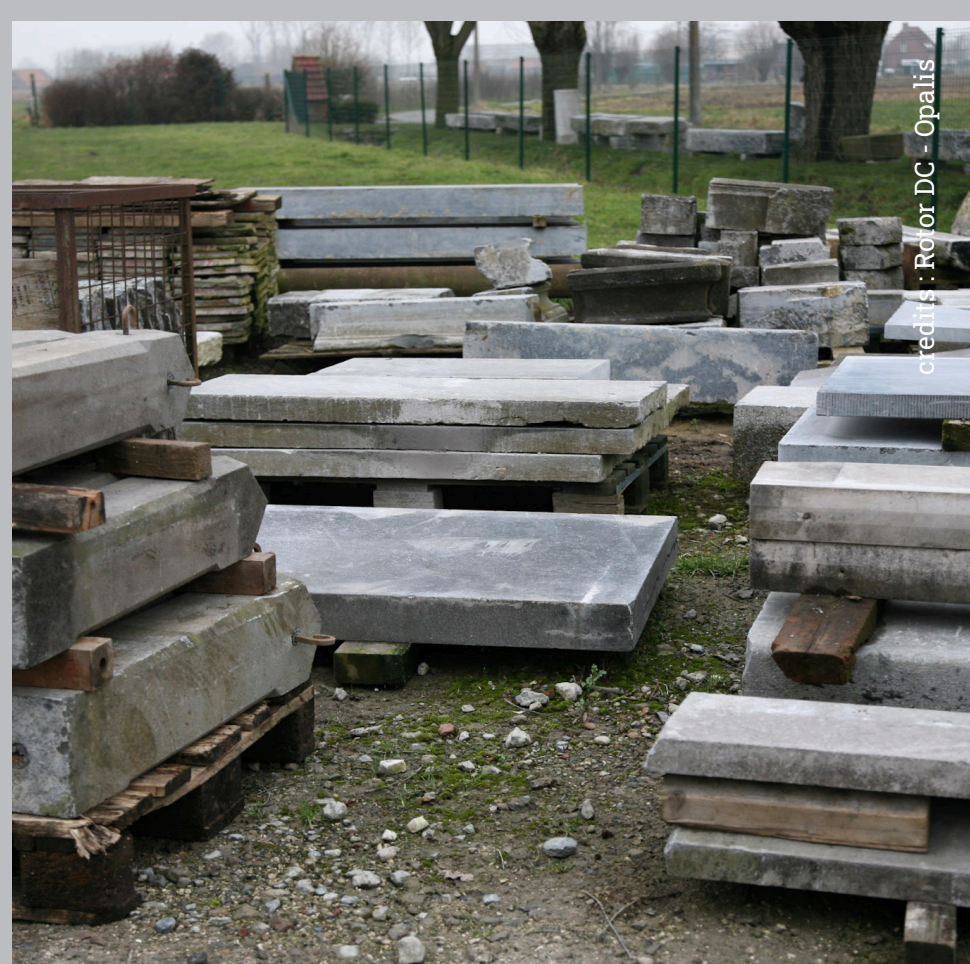
reclamation outlet of reusable sawn concrete blocks
